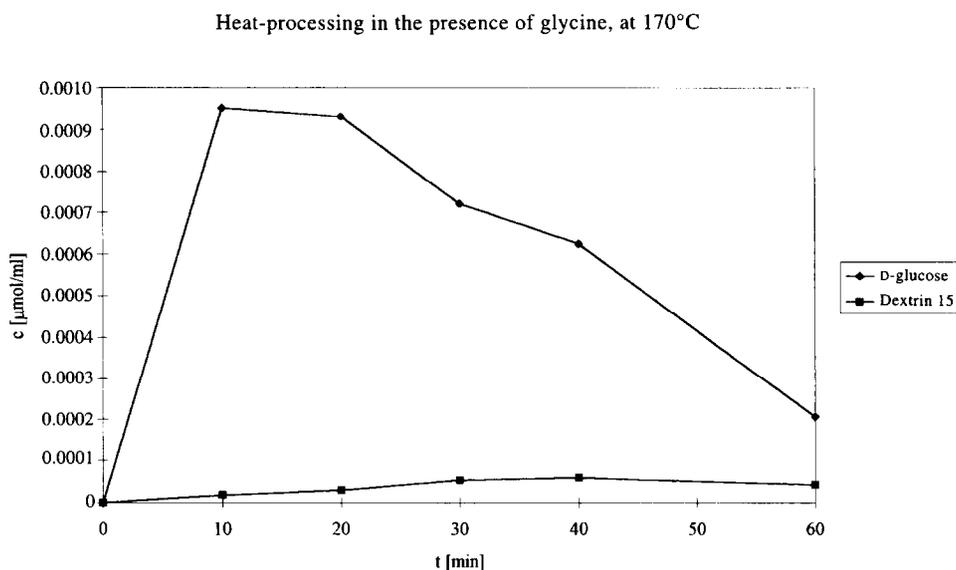
Fig. 8. D-glucose, dextrin 15 and starch caramelisation in the presence of glycine. Formation of methylglyoxal in aqueous solution vs. the period of heat treatment at 170°C.
