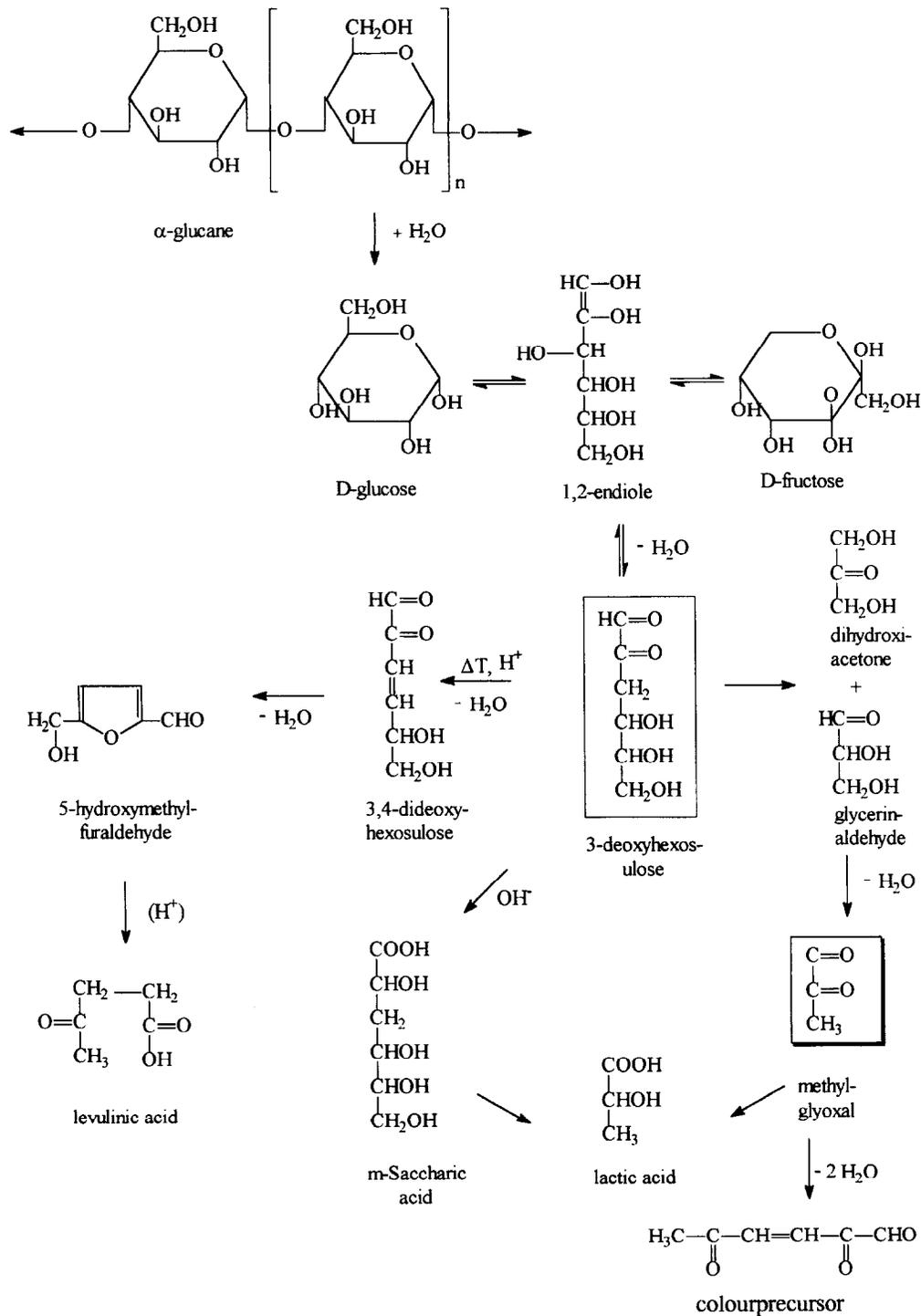
Fig. 1. Degradation of carbohydrates by caramelisation.
