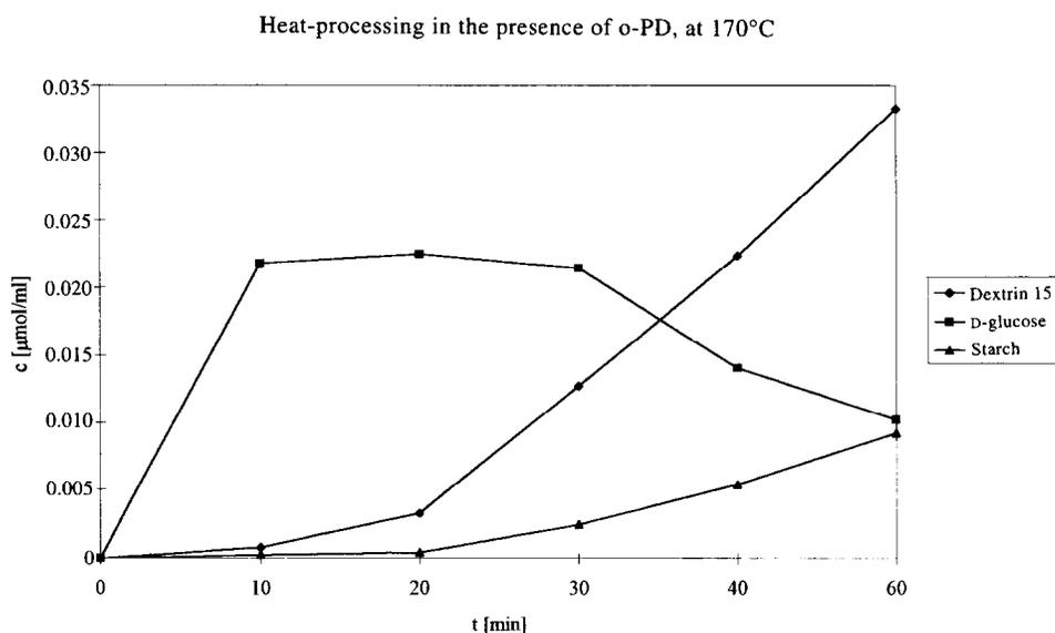
Fig. 7. D-glucose, dextrin 15 and starch caramelisation in the presence of o-phenylenediamine. Formation of methylglyoxal in aqueous solution vs. the period of heat treatment at 170°C.
