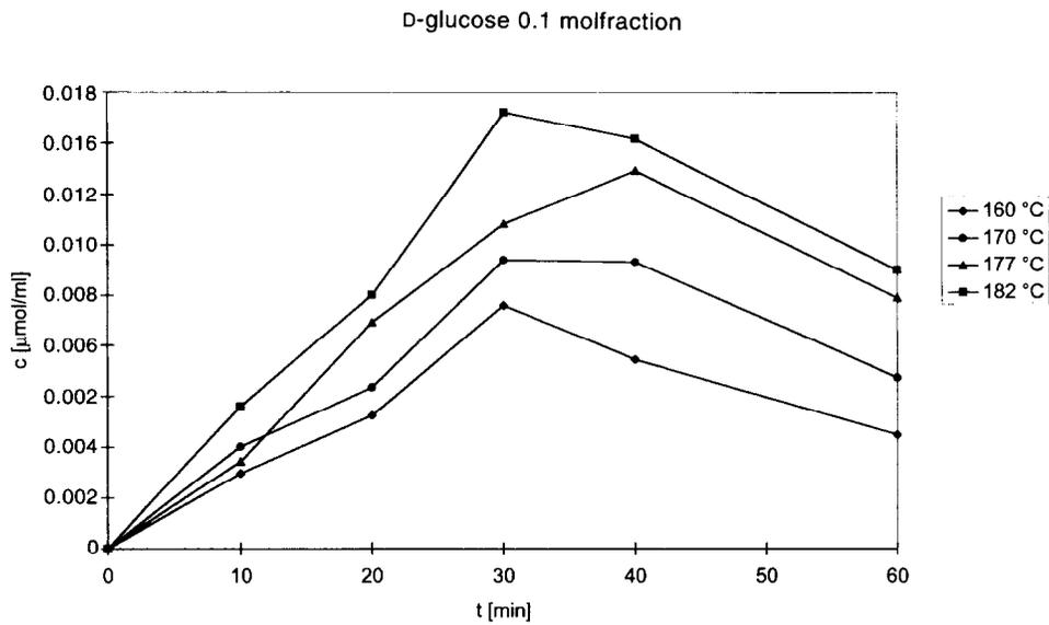
**Fig. 3.** Formation of methylglyoxal in 0.1 molfraction D-glucose caramel-solution vs. the period of heat treatment and different temperatures.
